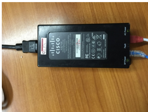
รูป 2 POE :Power Over Ethernet
